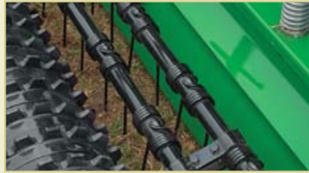
Tickler lines along entire working width incorporate and cover seed
