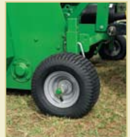
Optional front gauge wheels (cannot be used with optional front gauge roller)
